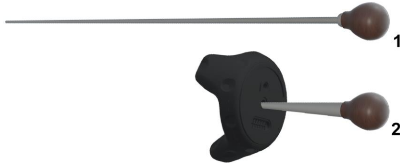
Fig. 3. The virtual baton models used in our user tests: 1) 3D model of a real conductor's baton, which was used in conjunction with the controllers A and B (Fig. 2) as test cases A1 and B1 respectively, 2) 3D model of the actual physical shape of our smart baton, which was used in conjunction with the controller B (Fig. 2) as test case B2.
