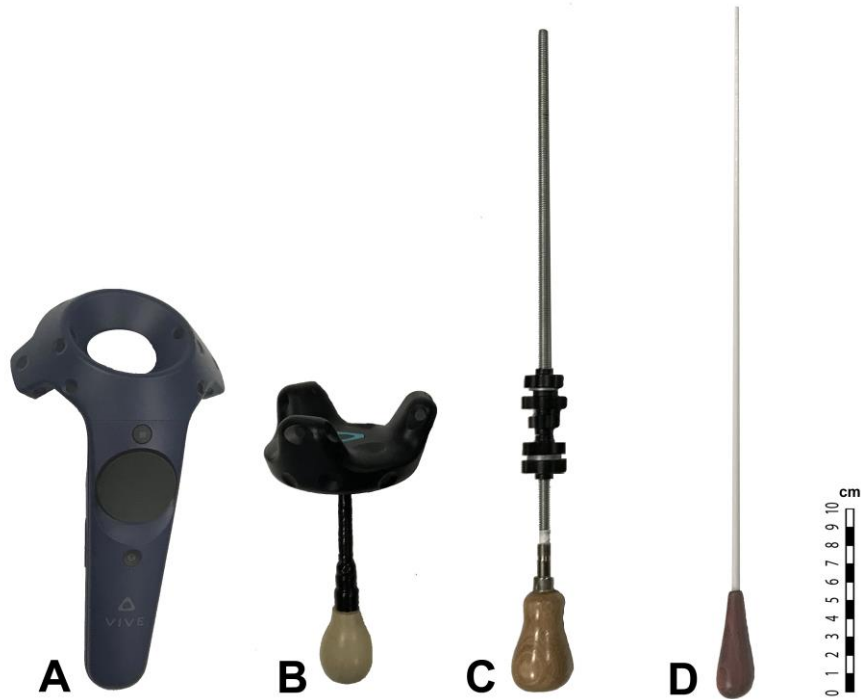
Fig. 2. A) HTC VIVE controller, B) Smart baton with VIVE tracker, C) Test baton with same weight as B, D) Real conductor's baton.
