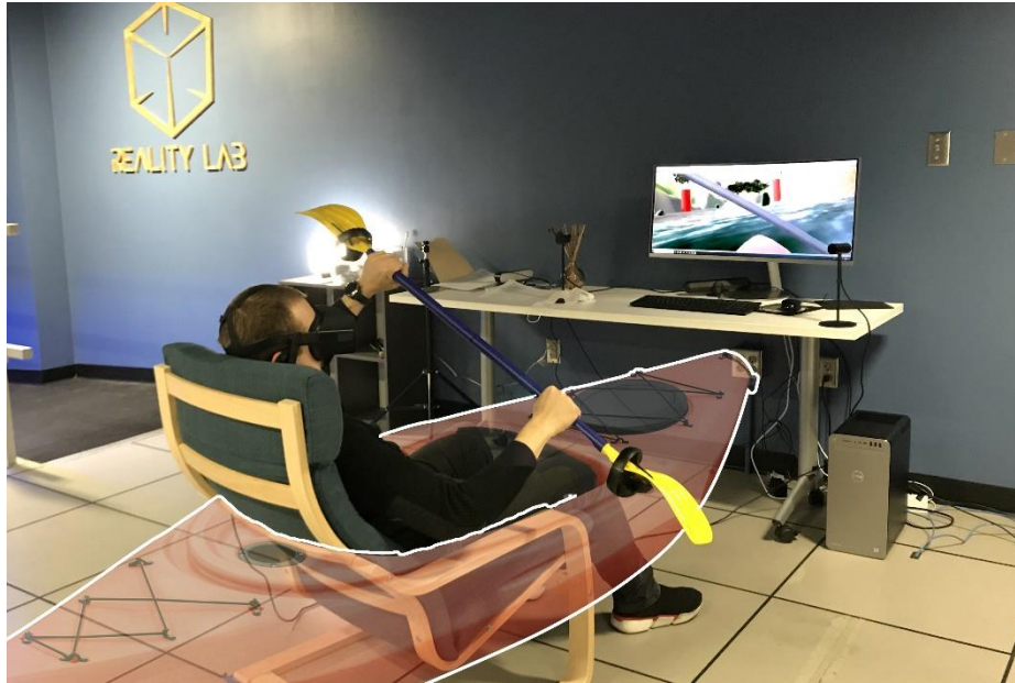
Fig. 2. The experimental setup in the Reality Lab of the Digital Worlds Institute. The virtual model of the kayak is superimposed to show the alignment between the real and virtual spaces.
