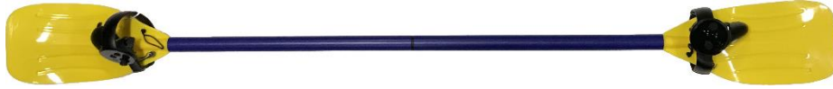
Fig. 1. The proposed “smart” paddle with the two VR controllers rigidly affixed to the two blades for 6-DOF tracking and vibration feedback when submerged in the virtual water.
