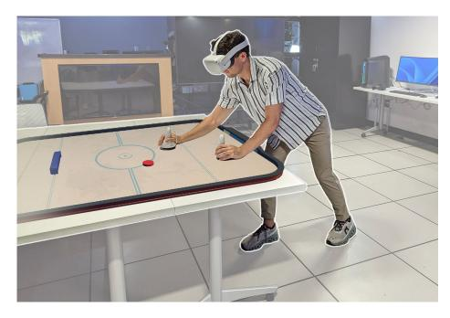
**Fig. 1.** Illustration of the experimental setup with a physical table. Components of the virtual environment are superimposed to show the alignment between the virtual and the real world.
