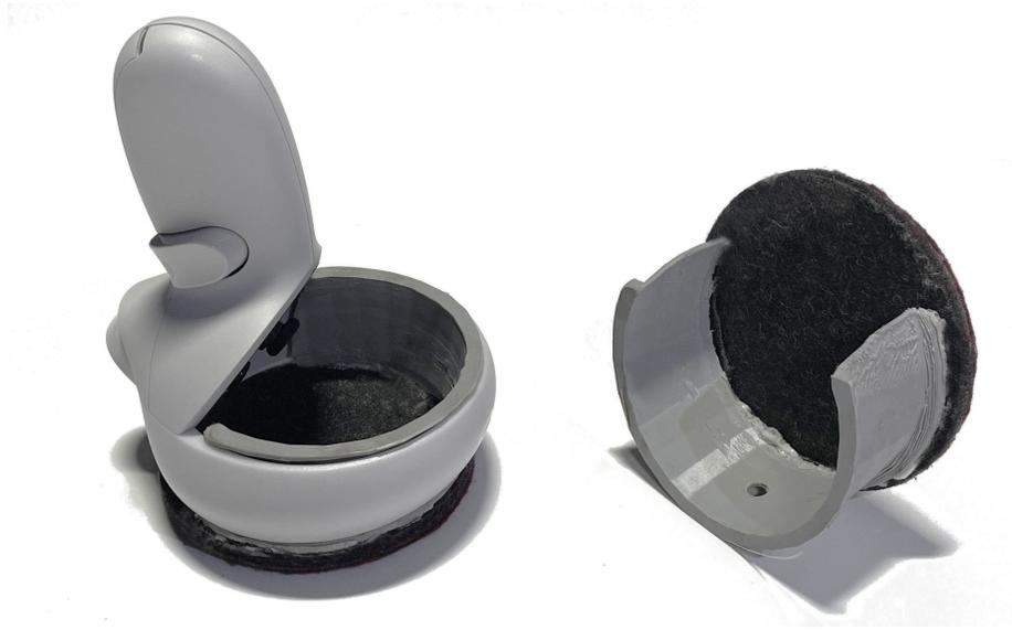
**Fig. 3.** Picture of the VR controllers with a 3D printed attachment and soft padding so that they can be used as air-hockey strikers on top of a physical table.
