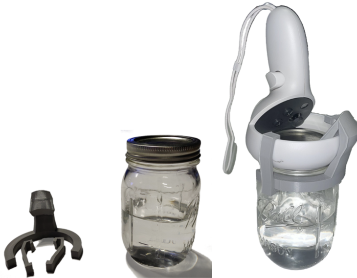
Fig. 3. Picture of the haptic jar with the VR controller using a 3D printed attachment.
