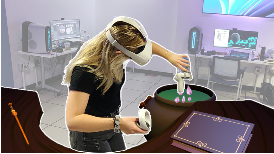
Fig. 1. Illustration of the user interaction using the physical jar. Components of the virtual environment are superimposed to show the alignment between the virtual and the real world.
