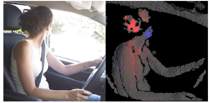
Fig. 8. An example of a video frame detecting intense head motion. On the right the corresponding computed directional magnitude of motion is shown in red or blue for increase or decrease of the depth values.
