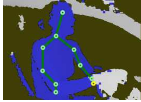
Fig. 3. Example of the skeleton model that was erroneously fit to an arbitrary frame of the depth sequence by the skeleton tracker provided with the Microsoft Kinect SDK.
