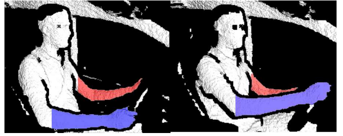
Fig. 5. Two examples of the proposed arm segmentation. Both arms can be clearly segmented from the rest of the depth frame even when one arm is occluded or partially visible from the depth camera (right).
