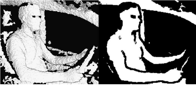
Fig. 2. Left: visualization of a depth frame. Right: The corresponding mask with enhanced boundaries between objects, computed using our framework.
