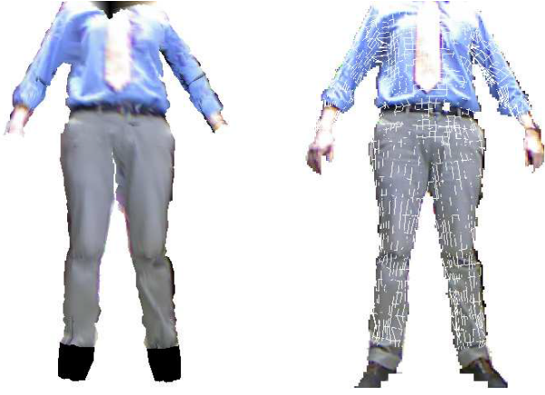
Fig. 4. Left: An intermediate state of the 3D reconstructed model before convergence. Right: The rectangular grid made of the current peaks of the data histograms superimposed on the current input frame in 3D.
