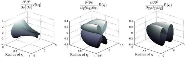
**Fig. 1.** 3D plots of three of the basis functions from Table 1. The functions were evaluated for varying  $\|\mathbf{q}\|$  over a unit circle of directions  $\mathbf{q}$ . The circle was defined by fixing the elevation spherical coordinate to  $\pi/3$  and varying azimuth.
