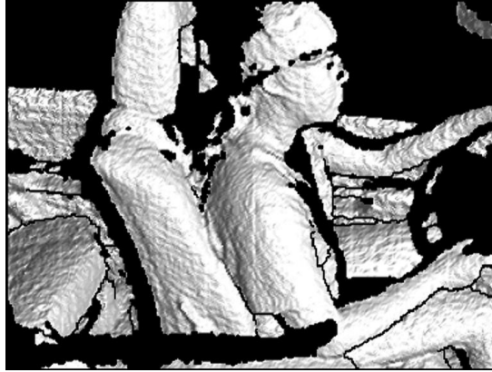
Figure 2: Example of a depth frame from the study dataset, visualized here as a 3D surface using computer graphics shading.
