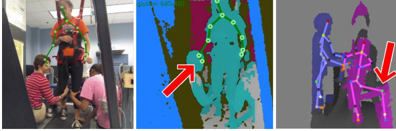
Fig. 5. Typical errors of existing skeleton fitting algorithms caused by the close proximity of the patient with other objects or human subjects in the clinical environment.
