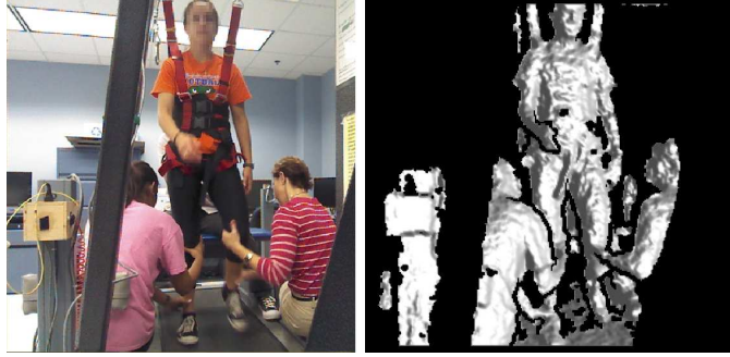
Fig. 1. A picture of our locomotor training environment (left), and the corresponding depth image (right) captured by a depth sensor located on the front of the treadmill.
