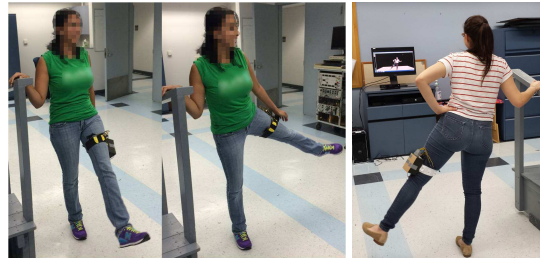
Figure 2. Test subjects following random vibratory cue-guided trajectories (left), and guided hip abduction exercises (right). The overall experimental setup is also shown, including the virtual training environments.
