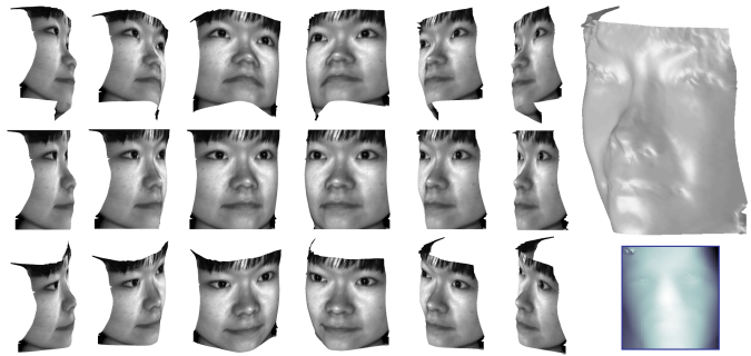
Fig. 11. Detailed pose variation with texture-less in upper right and depth-map in lower right. Photo-realistic renderings even in extreme poses can be noticed.
